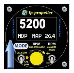
In this mode, the system adjusts the pitch completely automatically based on the MAP-RPM TARGET curve inserted in the microcontroller for the selected
