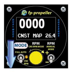
In this mode, the pilot decides the target RPM by turning the potentiometer (B) and the governor moves the propeller pitch to reach that target value. The Governor maintains that target value independently of the handle, within the limits set by the aircraft, the propeller and the flight conditions. The setting range for Rotax engines ranges from 4300 to 5800 RPM
